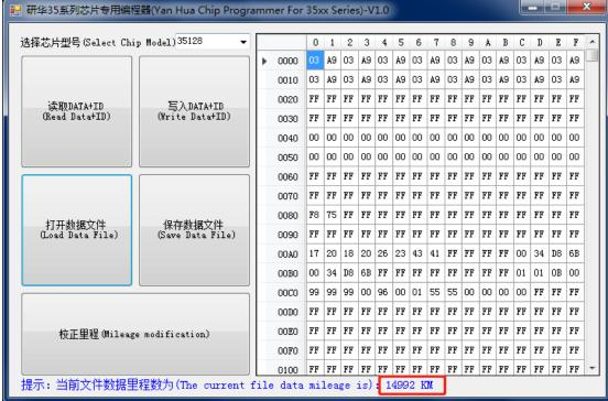
9. Once the mileage is confirmed, click "Write DATA+ID", Write the original data into the Simulator.
